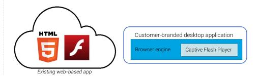
The Packaged Browser application works by loading in the appropriate browser engine and directing this to the predefined URL that hosts the web-based application. The browser engine then loads the custom version of the Flash® Player as provided under license by HARMAN. The web based application is then displayed as if it were running in a normal web page.
